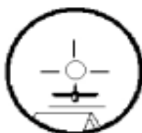
4. After firing, Aiming ring returns to centre until missile is gathered.
