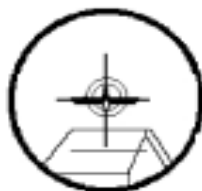
2. System switch ON, lay Aiming ring accurately over the target.
