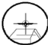
6. Re-lay crosswires on to target and continue to keep Aiming ring accurately using joystick.
