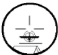
3. Press and hold Superelevation button and elevate until obstruction appears on Superelevation marker, keeping Aiming ring on target, release button.
